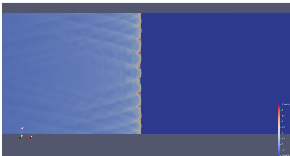
Fig. 3: Density field of two-dimensional H 2 detonation
